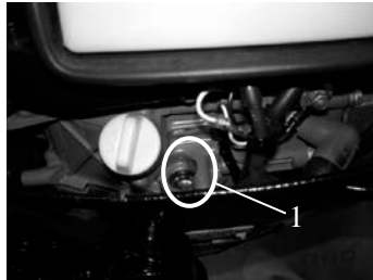
1.oil level check window
