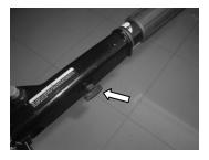
The throttle friction adjuster is on the tiller handle, which provides adjustable resistance to movement of the throttle grip, and can be set according to operator preference. To increase resistance, turn the adjuster clockwise. To decrease resistance, turn the adjuster counterclockwise. When constant speed is desired, tighten the adjuster to maintain the desired throttle setting.
