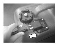
2. Connect fuel joints securely and squeeze the primer pump with the outlet end up until you feel it becomes firm .
