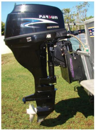
installed option to solve the problem of tilting the engine.
